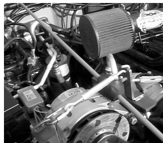
Belt tensioning system (turnbuckles, A210 bkt., link, & upright) (frnt. view)
