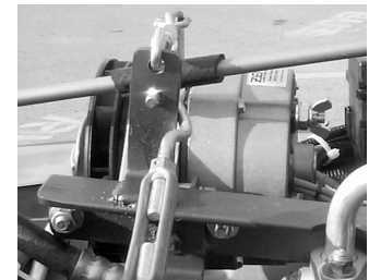
Detail of belt tensioning upright support (welded to bracket assembly) & bracket assembly
