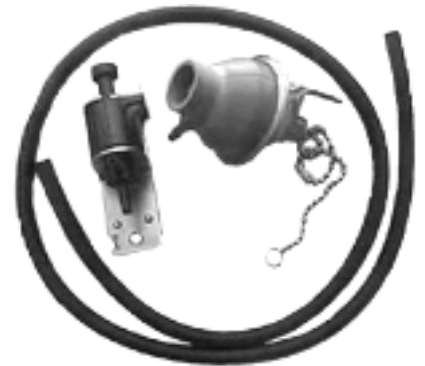
Automatic Engine Speed Control (when used in conjunction with control circuits built into all ZENA welders this accessory increases engine speed to optimum welding speed automatically when Power Button is depressed and returns engine speed to an idle as soon as Power Button is released) (for engines w/vacuum supply)
