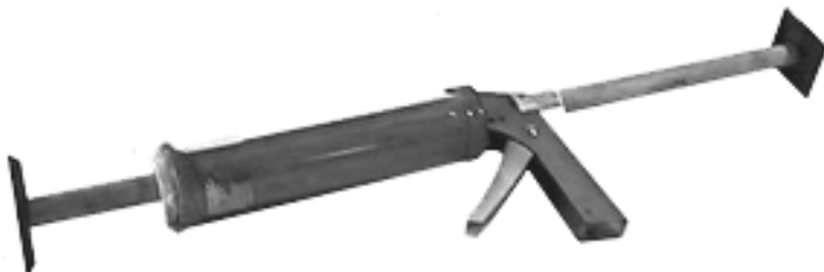
While not technically a bracket, this simple to build engine speed control mechanism made from scrap pieces of PVC pipe, a couple of furniture casters, and a caulking gun shows how a little ingenuity can make your welder easier to use.
